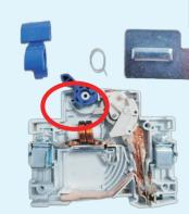
W4 Assembly of single stage multipole handle torsion spring, handle
